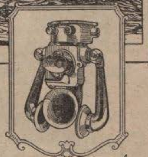
A typical Graham Patent Loud Speaking Naval Telephone as fitted in British Battleships.
